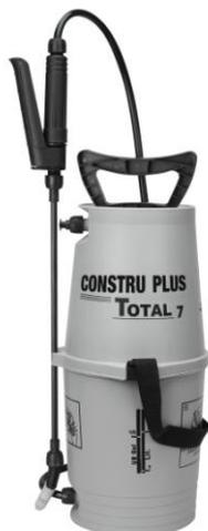
The constru plus 7 dual purpose injection cream pump and sprayer holds 5 ltr of injection cream, this saves time in changing cartridges or filling caulking guns ( see details for adapting to cream injection), this pump can also be used for timber treatment spraying, or spraying our range of block pave sealers.
